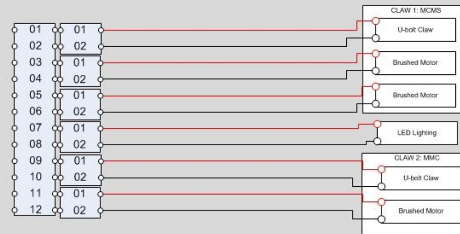
Accessory Motors 12 Conductor Pie Connector Female (Pins)
